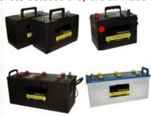
The starter battery is one that we are all familiar with under the bonnet of our vehicle. This type of battery is used to provide very heavy currents to a starter motor for short time periods. Because of this requirement, and thus its construction, it should not be deep cycled as its lifetime will be shortened as the plates will deteriorate rapidly.
